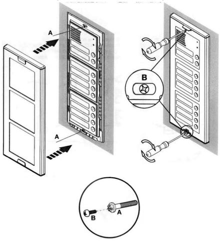
First screw on the bottom part of the frame. You can fit the frame into the fitting box 1145/5x system (original NUDV)
