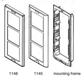
Removing the panel is done by extracting the fixing holders as per picture (on the side of the panel, in a forward direction)
