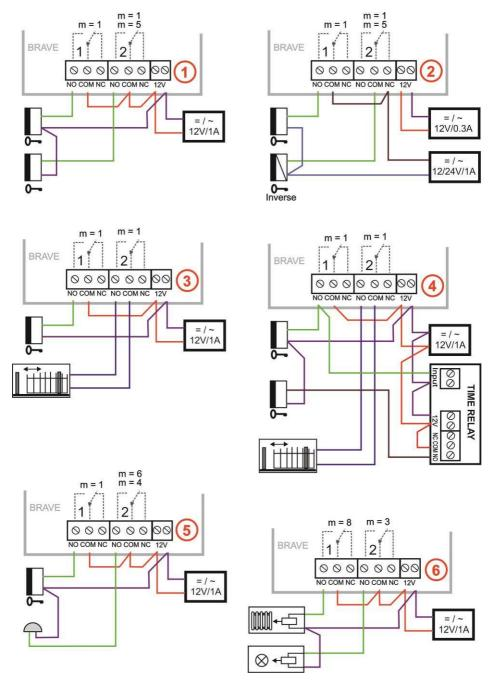
Pic. 4 Examples of relay connections
