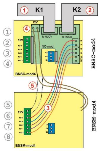
Pic. 2 Connection of BNSC-mod4 and BNSM-mod4
