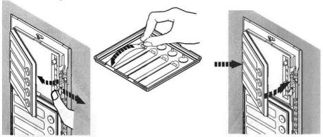
Paper tags are held to the front panel with a plastic holder. Follow the same procedure to place the panel back, being careful to insert the two lugs on the left carefully.
