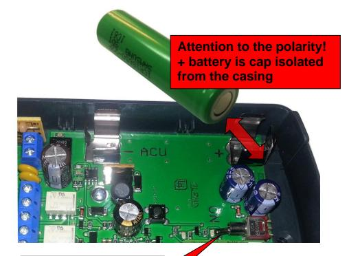
Before inserting the battery, off GDI using the switch (red LED goes out)
