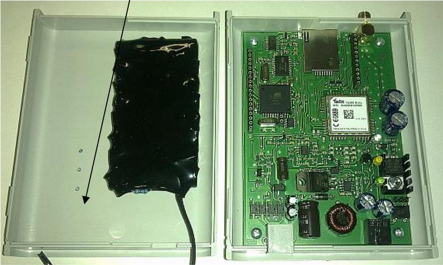
4. Batteries may not be supplied in a charged state. Turn on the gateway first, wait until it logs into the GSM network. Then connect the cable from the akupack to the connector.
