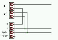
Selftest Input 1 (due relay A) – possibility activate Alarm remotely, Blocking Input 2 (due relay B) – Remote control of alarm circuit = Guarding for limited time
