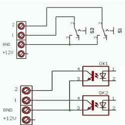
Connection with relay contacts, switches, magnetic contact switchers etc.
