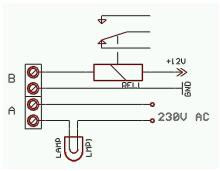
High power relay (clamper) connection, lightbulb connection (heating, engine etc.).
