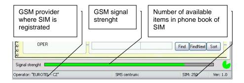
Program monitors communication microprocessor with GSM module. It shares this communication way to module. Microprocessor works with GSM module in 30 sec. period. It means that program has periodically 30 sec. For its own communication (loading or saving numbers) as same as SMS to SIM of the unit. This time is shown by green point in right program. Out down corner of of this time microprocessor works with GSM module) are some features unavailable.
