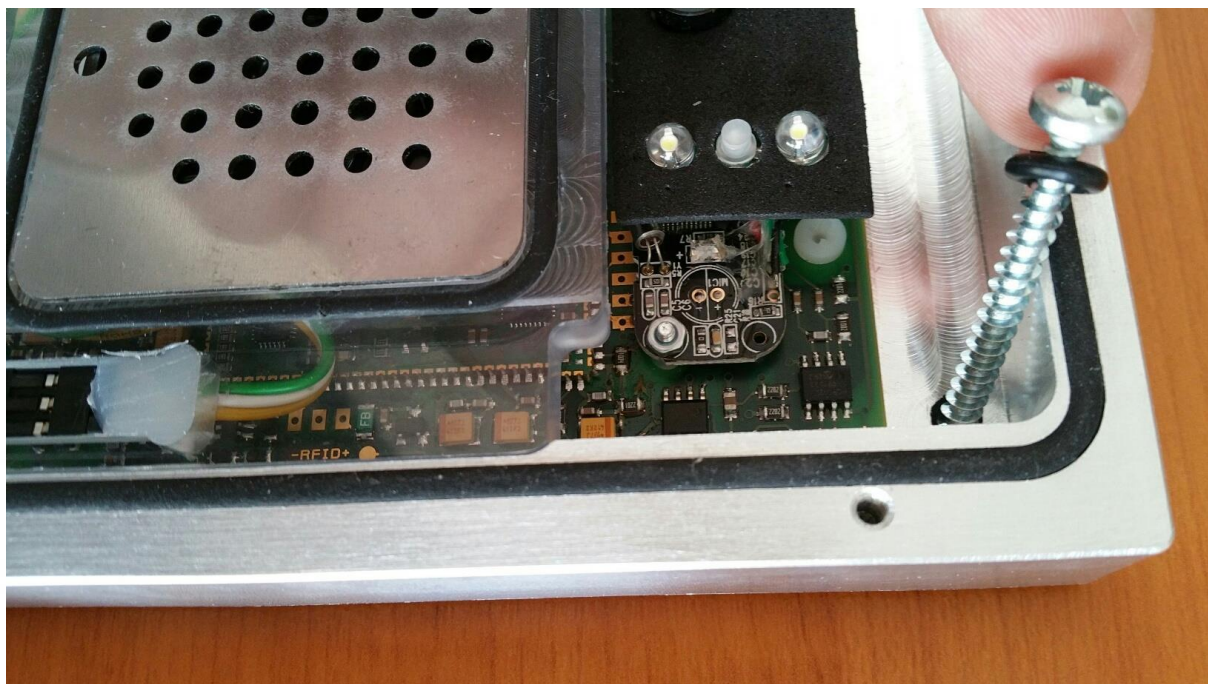
Fig 12. Use screws with rubber rings to avoid any leakages inside the unit
