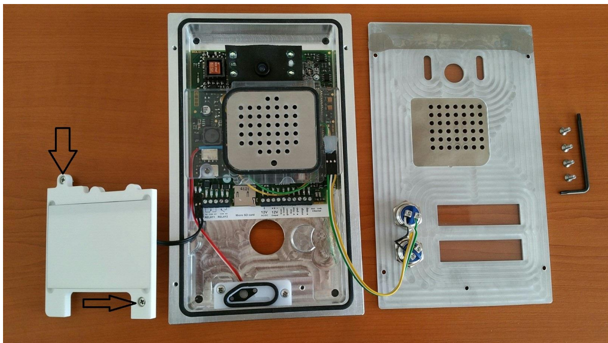
Fig 6. Using a cross head screwdriver, detach the top illuminated info module carefully (name/house number module). On the top front of the illuminated info module you can place your own label with your name, a house number or your required information, see Fig 19 for more details on changing the name plate.
