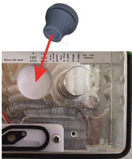
Fig. 7 Apply rubber bushing to avoid water leakages into the unit
