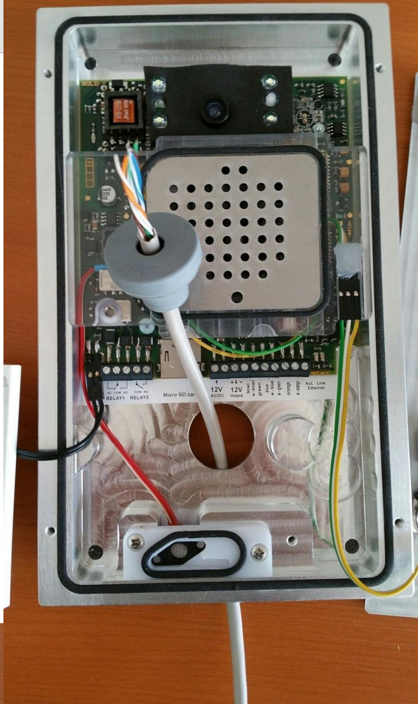
Fig 8. Use the rubber busing with IP67 impregnation rating to avoid any leakages inside the unit
