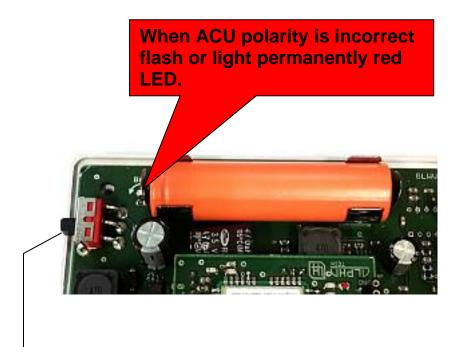
When all is correct then connect power supply and move switch to up position. – By this connect ACU into system.
