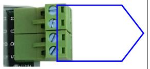
Screws for connection to ReMic module in lift cabin – connect same marked screws M – microphone G – ground
