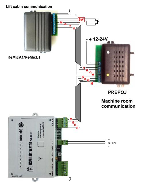
Connection example for communication lift cabin – shaft – machine room (totally possible connect 3pcs ReMic)
