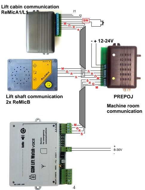
Connection example of activation by galvanically isolated screws of switch 12V ReMicA(L)1 – connection to bell or siren.
