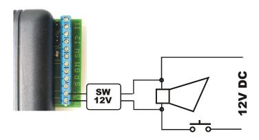
**Siren connection example in relay mode "button"** (Relay closed during button press)
