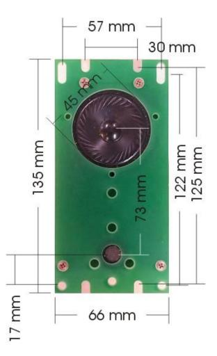
Fix the GSM part of unit either on lift cabin or in machine room. You have to select right place regards to GSM signal strength. Lift cabin installation is easier (it is not necessary cable from lift cabin to machine room and due this is avoid of interference). However you have to provide good signal strength for all lift shaft! Keep in mind enough manipulation space for SIM card.
