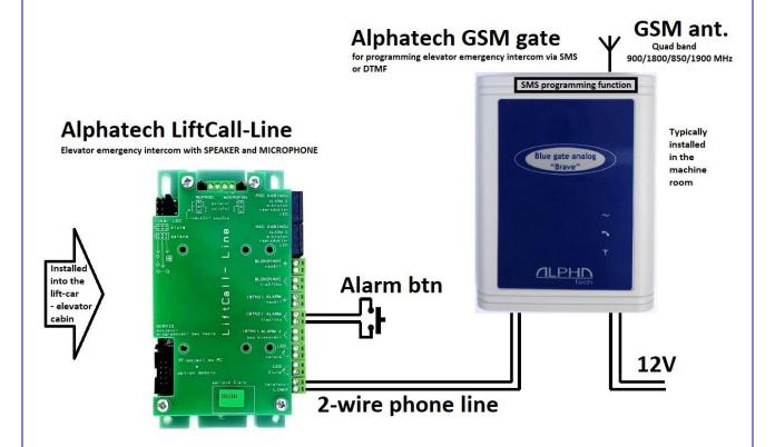
The SMS text message is sent to the GSM gateway phone number: DTMF cc,c...,...cc
