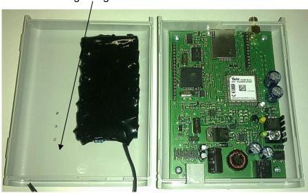
4. Batteries may not be supplied in a charged state. Turn on the gateway first, wait until it logs into the GSM network. Then connect the cable from the akupack to the connector.
