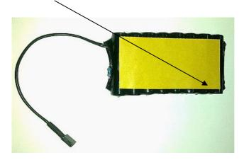
3. Fix the ACU pack into Gateway cabinet. CAUTION for holes for signalling LEDs! DO NOT COVER!
