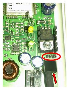
state. Start the gateway first and wait for network log in. Then connect cable from ACU pack to appropriate connector...
