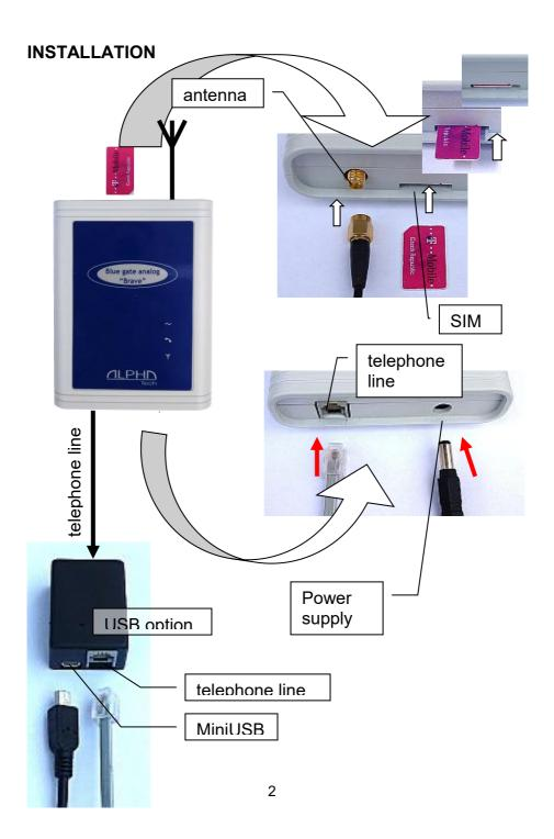
Insert the SIM card up the picture and by press fix it in operation position. Before inserting the SIM card we recommend checking at various mobile phone state of the SIM card (logging with or without PIN, PIN, etc.) and set logging without PIN. When you want logging with PIN you have to preprogrammed this PIN and set logging with PIN (via table of programming). Without this setting the Gate wont work.
