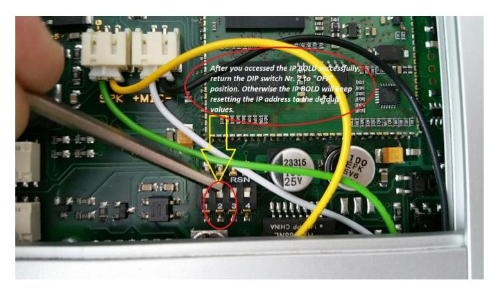
Please do not forget to return DIP switch Nr. 2 to "OFF" position after you accessed it via web interface. In "ON" position it will keep resetting the IP BOLD doorphone, keeping its default IP address 192.168.1.250.
