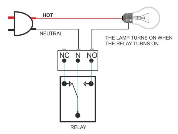
The above image shows a basic connection diagram that can be used in most situations. The connection diagram is the same for both AC and DC loads. Please make sure to use a freewheeling
