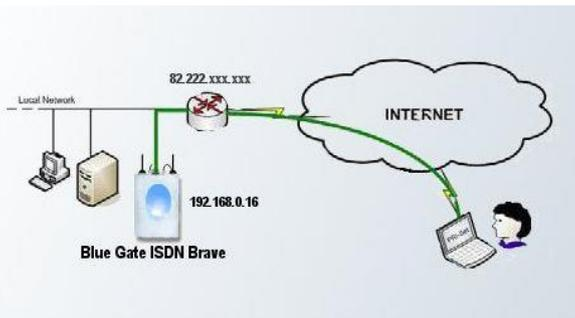
BRI Gate can be programmed remotely via Internet. This is possible by VPN access or port forwarding on router.
