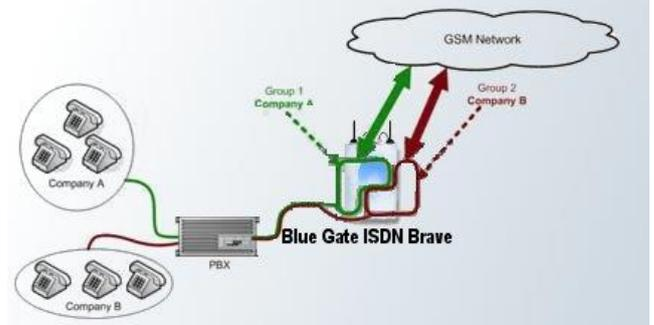
The gateway Blue Gate ISDN Brave is able to analyse dialled number and forward the call through GSM Network or PSTN BRI access. Also, if both GSM/UMTS modules are busy, it is possible to forward the call through PSTN BRI network. Calls coming through PSTN BRI access are forwarded directly to the PBX.
